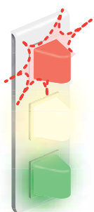
The red indicator flashes and the green and white indicators remain on with a steady light.
