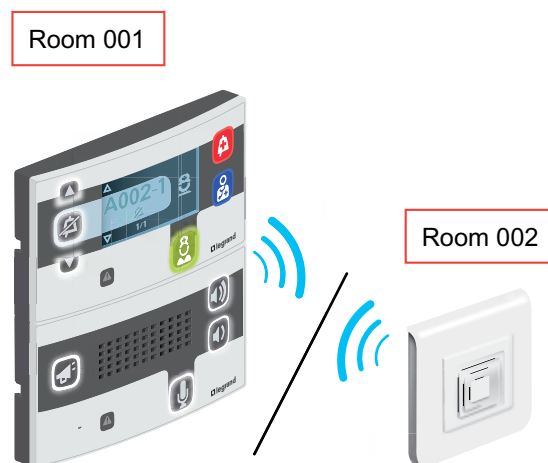
The nurse makes contact with the patient. The audible alarm is cut off.
