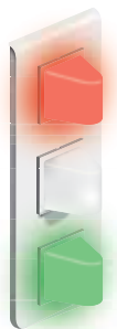
The red and green indicators on the corridor light unit come on with a steady light.
