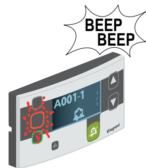
The nurses' station control unit signals the room making a call and emits a more rapid audible alarm.
