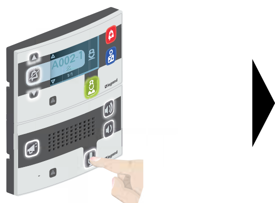
Once the conversation has finished, if the nurse needs to go to room 002, they simply cut interphone communication.
