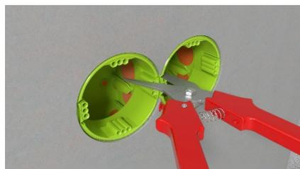
If necessary, the SCS connecting bar can be cut out.
