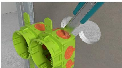
Open the membrane with the cutter knife and insert the pipes without tools.
