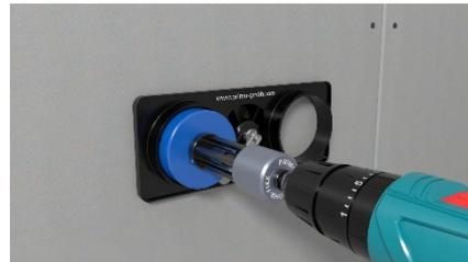
Optional: Mill out additional drill holes with the drilling template (P102-74) to save time and ensure accurate measurements.
