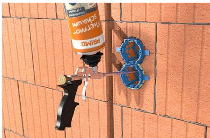
Insert can, spray foam = installed in a few seconds, free of thermal bridges and airtight.
