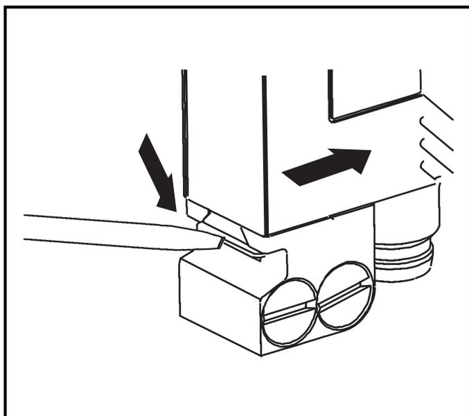
To remove the unit press the spring down with a screwdriver and slide the unit out.
