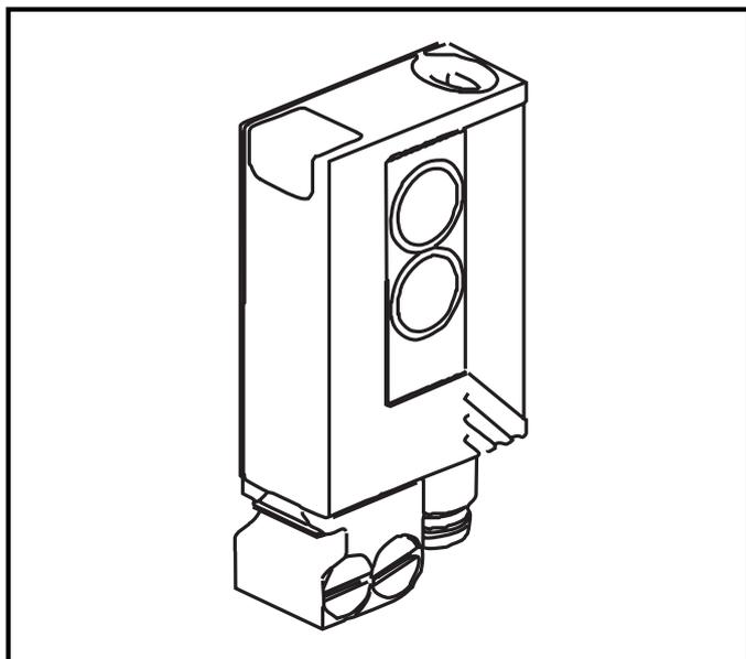
Secure the mounting fixture with the screws supplied, then slide the unit into the slot of the fixture until the spring clicks home.
